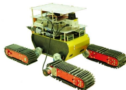
Fig. 1: A four wheeled skid-steered UGV.
